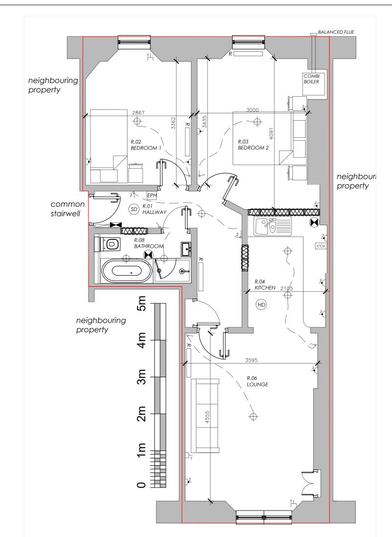
proposed floor plan 1:50 @ A3 (Air B'n'B use)
